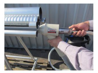
If the heat exchanger tubes are not too dirty (short cleaning cycles) it is an alternate to work without Y fitting.
